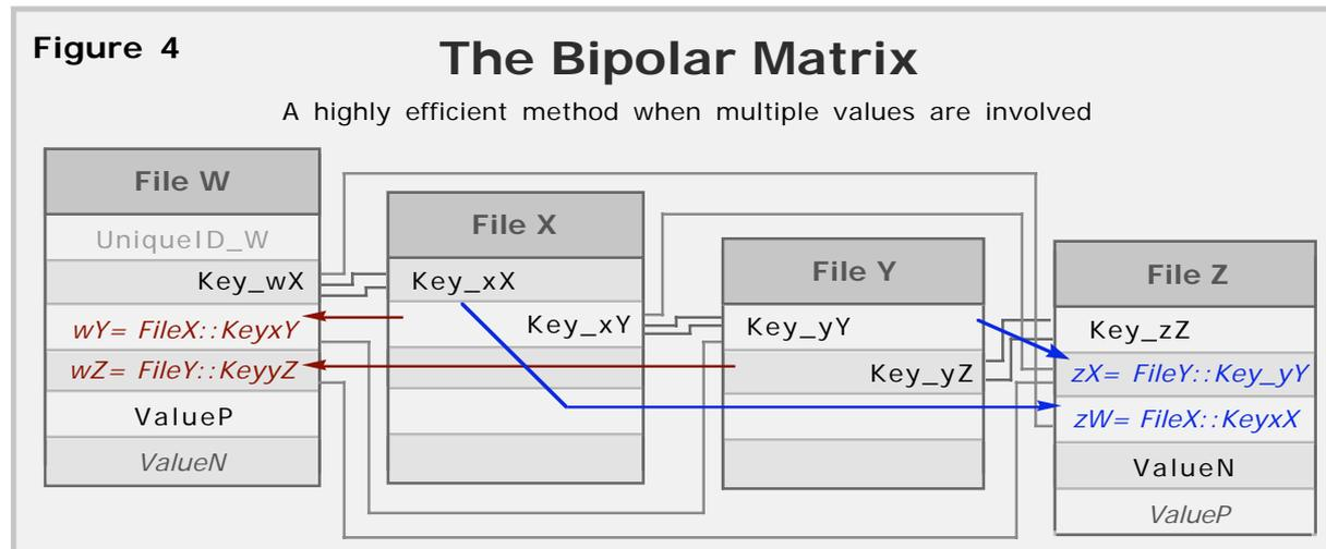
Thus a three dimensional logical 'data map' can be assembled, based on a network of unstored key fields, through which related data can be drawn directly to any point in the data flow via a single step data call (based on the matrix key system) rather than via lengthy lines of data shunts.
