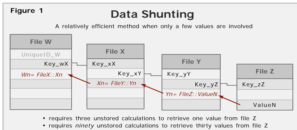
Data shunts may do the job relatively effectively when the number of fields is small. As indicated on the diagram, the number of unstored calculations required is a multiple of the number of values to be retrieved and the number of files between the source and destination. This potential deluge of unstored calculations can be cumbersome and inefficient - and may also make it difficult to focus on the true role and purpose of the data within each file in a solution.
